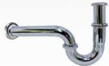
BBT-3202 32mm CP Brass Tubular Trap Outlet Pipe : L330mm Vertical Pipe : L180mm
