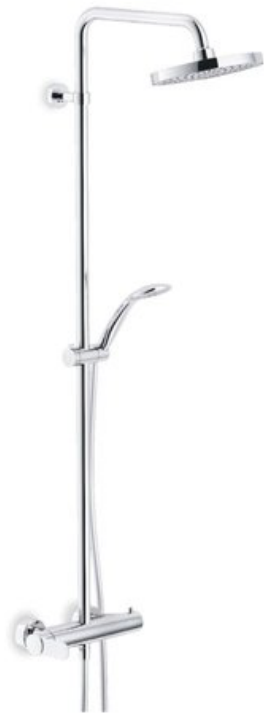
SA99130/30CR External single control mixer, swivel shower head ø 200 mm with rain jet, single jet shower head
